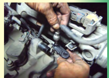
A2218 use on Injector Tube Fitting
