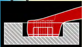
Deeper Accessibility Ring Head provides better accessibility in confined areas
