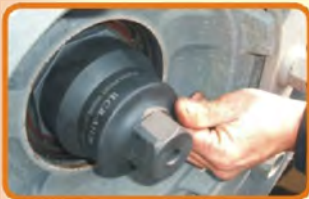
B1125 Front Wheel Socket Remove axle lock nut
