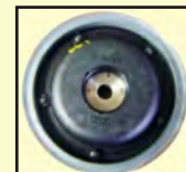
A1276 Groove nut socket to turn the camshaft adjuster into position.
