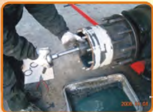
A1278 Axle Hub Nut Socket Adjust axle bearing nut
