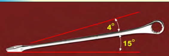
Picture show 15° offset with Open-End parallel to nut
